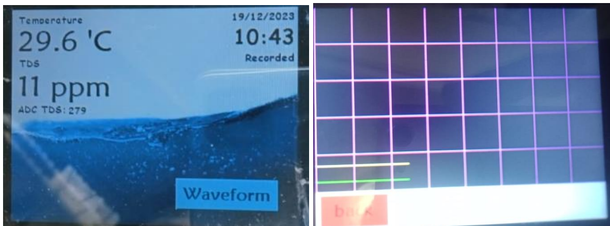
Figure 3. TFT displays images showing salinity and solution temperature measurement results in real-time numbers and curves
