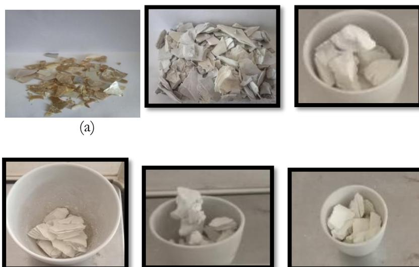
**Figure 2.** Calcination results of clam shells (a) Before calcination (b) calcination temperature of 750°C, (c) calcination temperature of 800°C, (d) calcination temperature of 850°C, (e) calcination temperature of 900°C, (f) calcination temperature 950°C.
