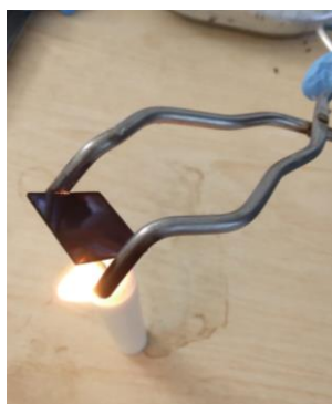
Figure 5. counter electrode Coating with Carbon
