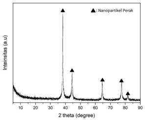
Figure 4. XRD Characterization of Silver Nanoparticle
